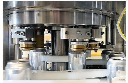
The CB100R counter-pressure canning line employs a 12-head rotary filling turret, coupled with a 3-spindle rotary seamer, to allow the machine to fill more than 100 CPM. The full rotary, continuous motion design ensures the smooth transition of cans through the system at higher speeds, effectively limiting agitation that can reduce product quality.
